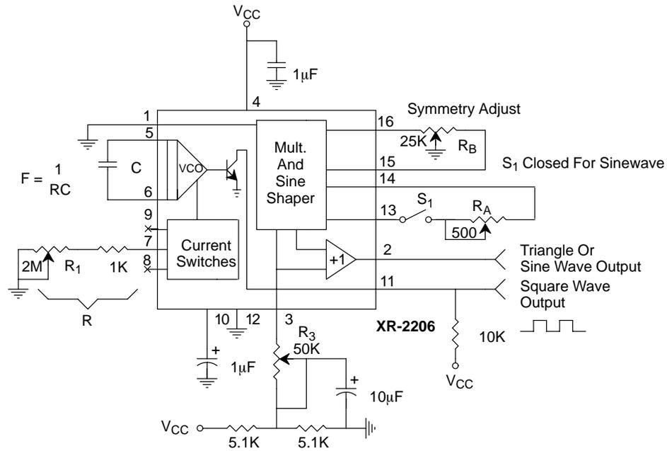
Figure 12. Circuit for Sine Wave Generation with Minimum Harmonic Distortion. (R<sub>3</sub> Determines Output Swing - See Figure 3)
