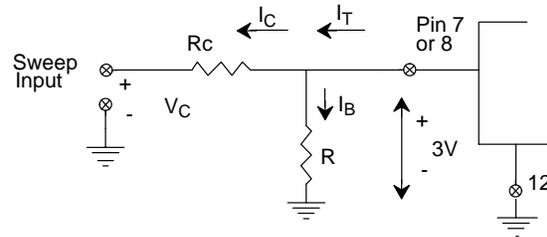
**Figure 10. Circuit Connection for Frequency Sweep.**
