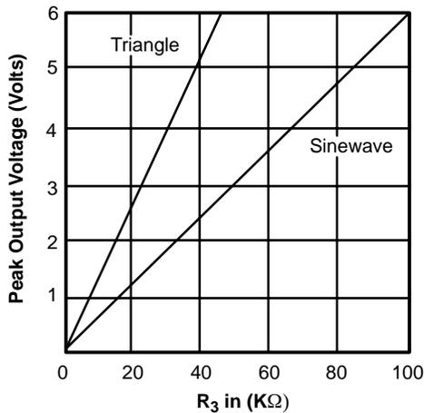
Figure 3. Output Amplitude as a Function of the Resistor, R<sub>3</sub>, at Pin 3
