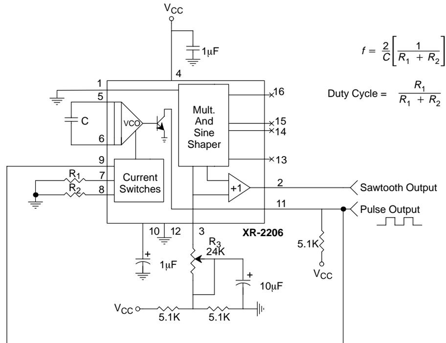
**Figure 14. Circuit for Pulse and Ramp Generation.**
