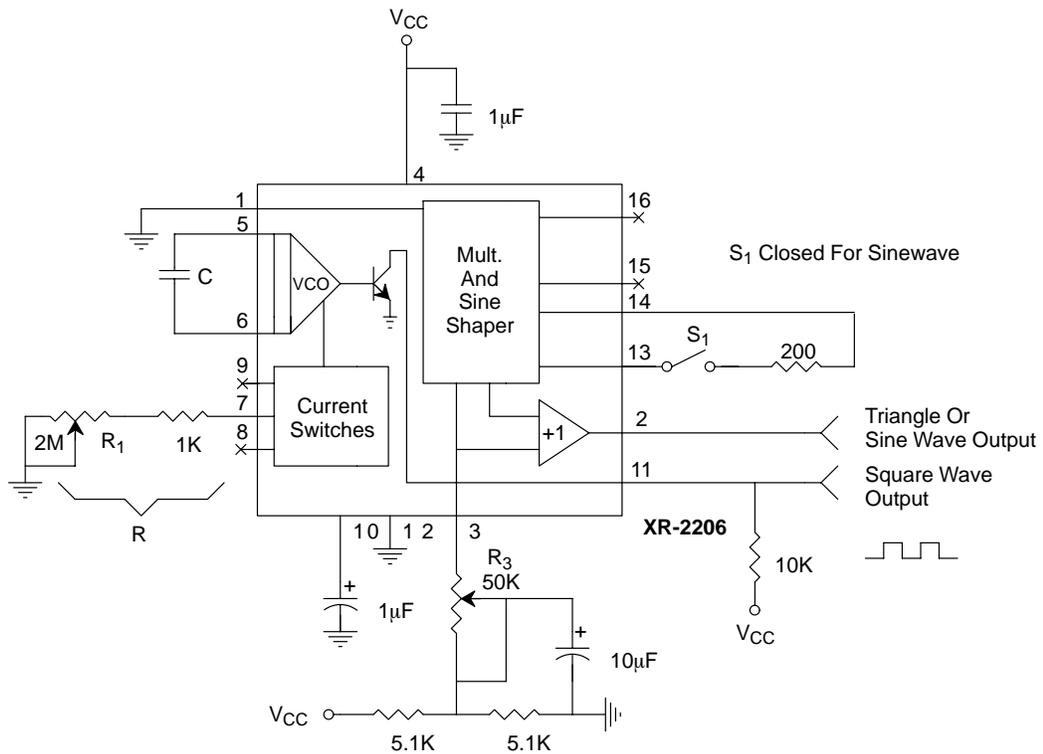
**Figure 11. Circuit for Sine Wave Generation without External Adjustment. (See Figure 3 for Choice of R<sub>3</sub>)**
