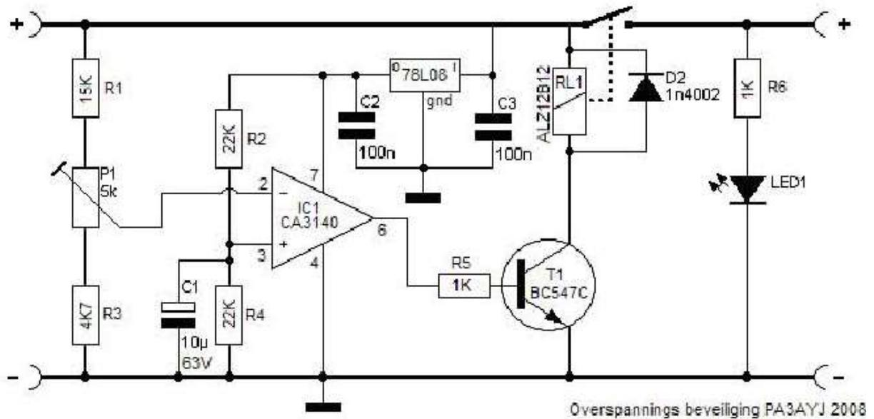
Switching transistor T1 (for example BD135) for switching car relays (with larger coil current)
